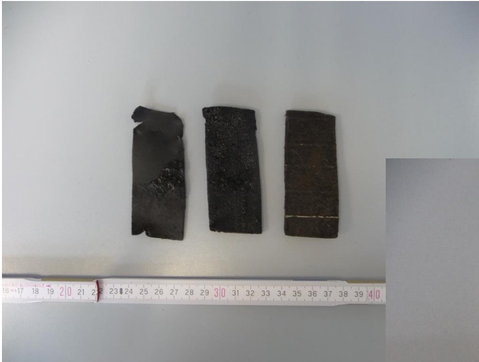
Dachpappe (Asbest)
